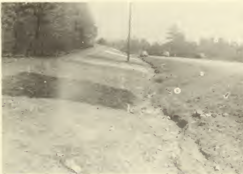
Figure 24.--A general view (in upper half of photograph) of roadside areas sown to common bermudagrass, with different plots mulched with pine straw, 2 and 4 tons per acre of grain straw, paper mesh, clear plastic and no mulch. Mulch was essential for anchoring seed and fertilizer on steep slopes and for protecting all slope conditions from heavy rainstorms. In general, the crop straws were more effective and easier to use.
